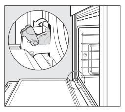
■ To release the locking clamps on the hinges. See illustration.
